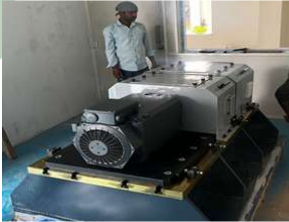
Fig. 10.1: Dynamometer with Battery Emulator (30 kW)
