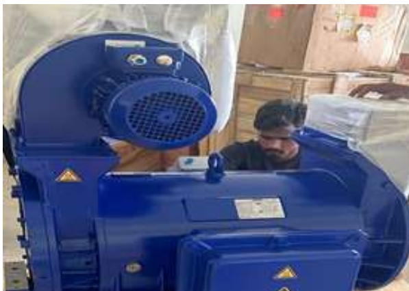
Fig. 10.2: Dynamometer with Battery Emulator (150 kW)
