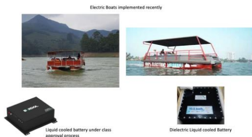
Figure 92 Marine boats re-fitted with Yesen Sustains Electric conversion kit and their battery systems
