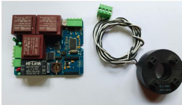
Figure 86 Clamp-on CT based Wireless Energy Meter Board developed by Tranquility
