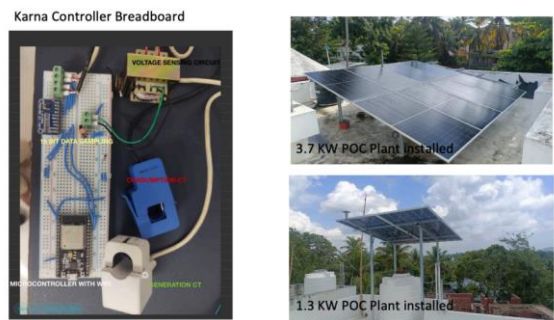
Figure 89 MistEO Pvt Ltd - Installation of the demo plant in Trivandrum and prototype of the controller
